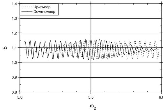
Fig. 11. Drop equatorial radius as a function of the instantaneous modulation frequency  $\omega_2(t)$ . Still we take  $S = 3.757$ ,  $\kappa = 1.055$ ,  $B_a = 1.00$ ; the modulation amplitude is  $\varepsilon = 0.01$ , the sweeping rate  $d\omega_2/dt = \pm 3.1535 \times 10^{-2}$  starting from  $\omega_{20} = 5.036$  for the up-sweep and  $5.980$  for the down-sweep, respectively.
