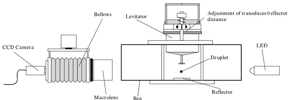
Fig. 1. Sketch of the experimental apparatus.
