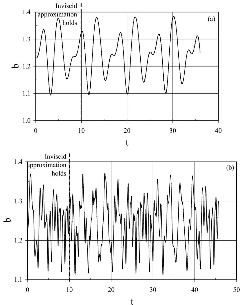
Fig. 6. (a) The equatorial radius as a function of time for  $\kappa = 0.575$ ,  $B_a = 2.15$ ,  $\varepsilon = 0.05$ , and  $\omega_2 = 1.5$ . A pattern of  $\Delta t = 8.57$  is repeated several times virtually without modifications, a quasi-periodic case. (b) The equatorial radius as a function of time for  $\kappa = 0.575$ ,  $B_a = 2.15$ ,  $\varepsilon = 0.20$ , and  $\omega_2 = 5.66$ . No periodicity at all can be recognized any more.
