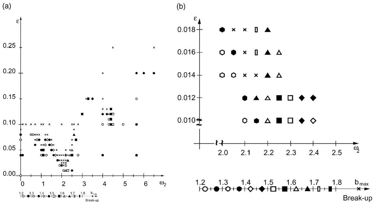
Fig. 5. Parameter configurations ( $\varepsilon$ ,  $\omega_2$ ) that lead to drop break-up are marked by a cross; configurations that lead to drop oscillations are labelled by a symbol that indicates the maximum equatorial radius  $b_{\max}$  during the oscillation. Fig. 5b is an enlarged detail from Fig. 5a; it can be concluded that the first drop eigenfrequency  $\omega_2^{(\text{res})}$  decreases with increasing modulation amplitude  $\varepsilon$  or oscillation amplitude.
