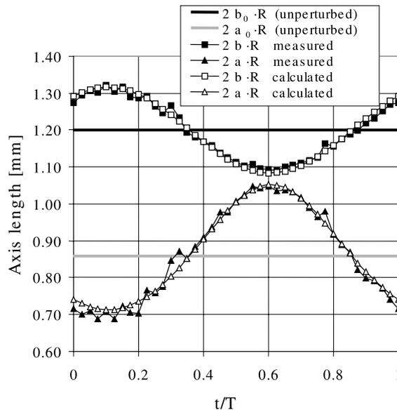
Fig. 7. Comparison between measured and calculated length of the dimensional major axis  $2bR$  and minor axis  $2aR$ . The period of oscillation was about  $T = 12.5$  ms, which is quite close to the value of 13 ms following from Eq. (1). The same drop as in Fig. 2;  $\varepsilon = 0.005$ ,  $\omega_2 = 5.0307$  (rendered dimensionless by  $(g/R)^{**} (1/2)$ ).
