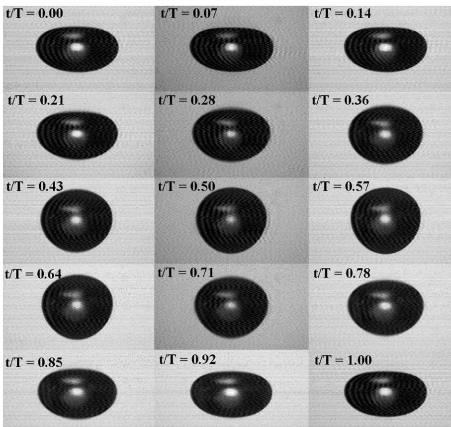
Fig. 2. Images of an *n*-hexadecane droplet in the mode  $l = 2$  (dimensional volume  $5.18 \mu\text{l}$ ,  $b/a = 1.4$ ) at different states of deformation.  $T = 12.5 \text{ ms}$  represents the period of one full droplet oscillation. Maximum oblate deformation is at  $t/T = 0.07$  and maximum prolate deformation is at  $t/T = 0.57$ .
