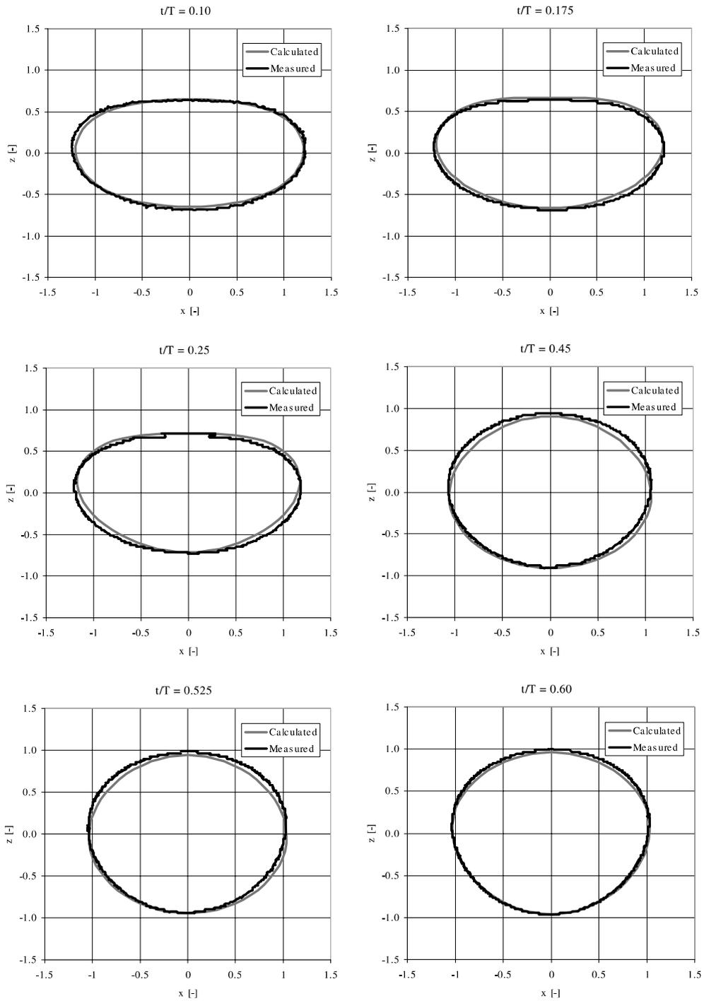
Fig. 8. Comparison between measured and calculated droplet shapes at different deformation stages. The dimensionless time  $t/T$  is given in each diagram. The coordinates  $x$  and  $z$  are rendered dimensionless by the radius of a volume equivalent sphere. The same drop as in Fig. 2;  $\varepsilon = 0.005$ ,  $\omega_2 = 5.0307$  (rendered dimensionless by  $(g/R)^{**} (1/2)$ ).
