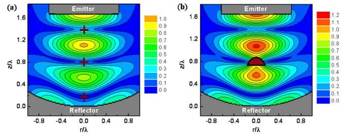
FIG. 2. (Color online) Distribution of the sound pressure field: (a) before the levitation of ladybug and (b) during the levitation of ladybug. The sound pressure at the center of the emitter surface is  $p_0=3560.8$  Pa (SPL = 162 dB) before levitation. The coordinates  $r$  and  $z$  are scaled by the wavelength  $\lambda=20.3$  mm, and the sound pressure  $p$  is scaled by  $p_0$ . The cross “+” in (a) indicates the pressure minima which are the possible levitation positions.
