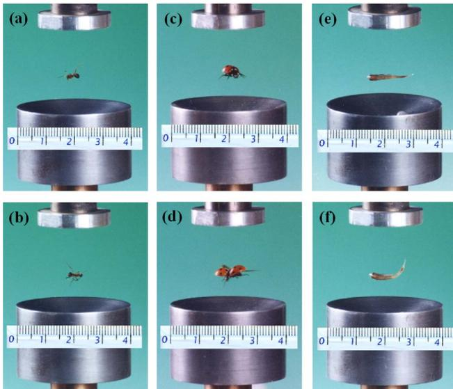
FIG. 1. (Color online) Acoustic levitation of small living animals in air: [(a) and (b)] ant, [(c) and (d)] ladybug, and [(e) and (f)] young fish. The ruler scale in [(a)–(f)] is cm.
