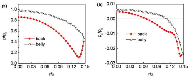
FIG. 3. (Color online) Distribution of (a) sound pressure  $p$  and (b) acoustic radiation pressure  $p_a$  on the ladybug's back and belly. The reference pressure  $p_0=3560.8$  Pa (SPL=162 dB) is the sound pressure at the emitter center.
